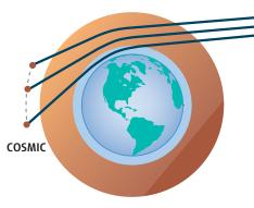
Locked on. Cosmic satellites (blue, right) track signals from GPS satellites (beige, right) and log how the atmosphere bends them (above)data that reveal temperatures.
