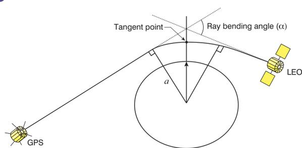
Figure 1 Illustration of the GNSS-RO geometry and the impact parameter 'a'.
