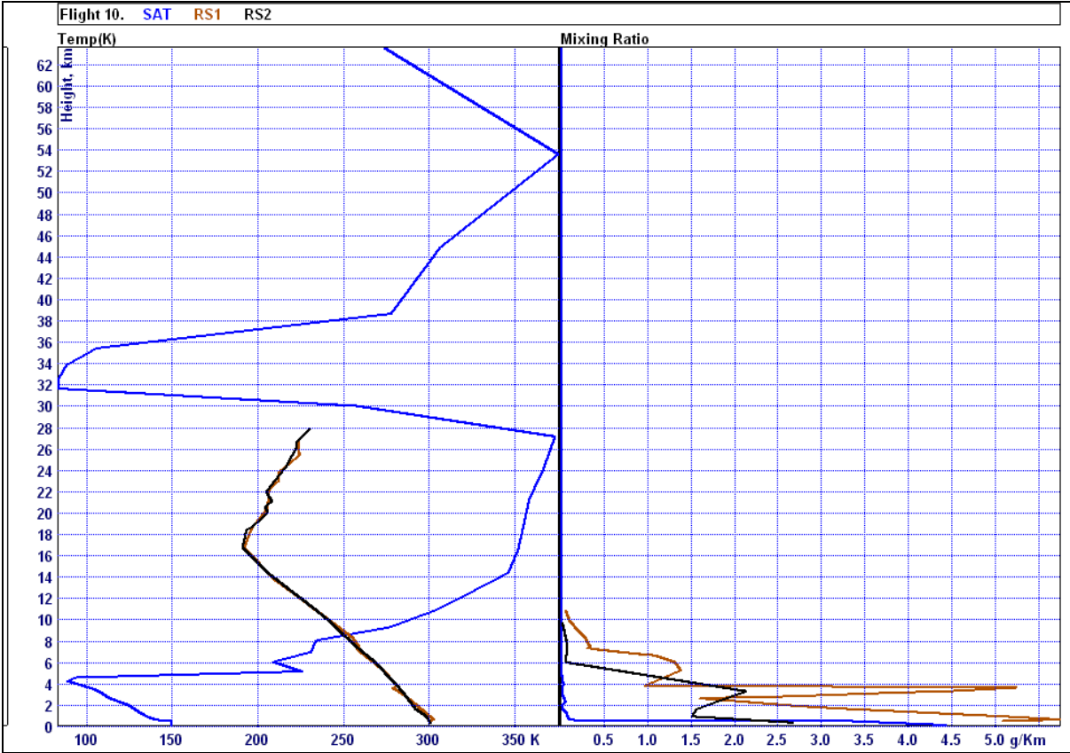
Figure E1 Comparison 10's erroneous satellite profile
