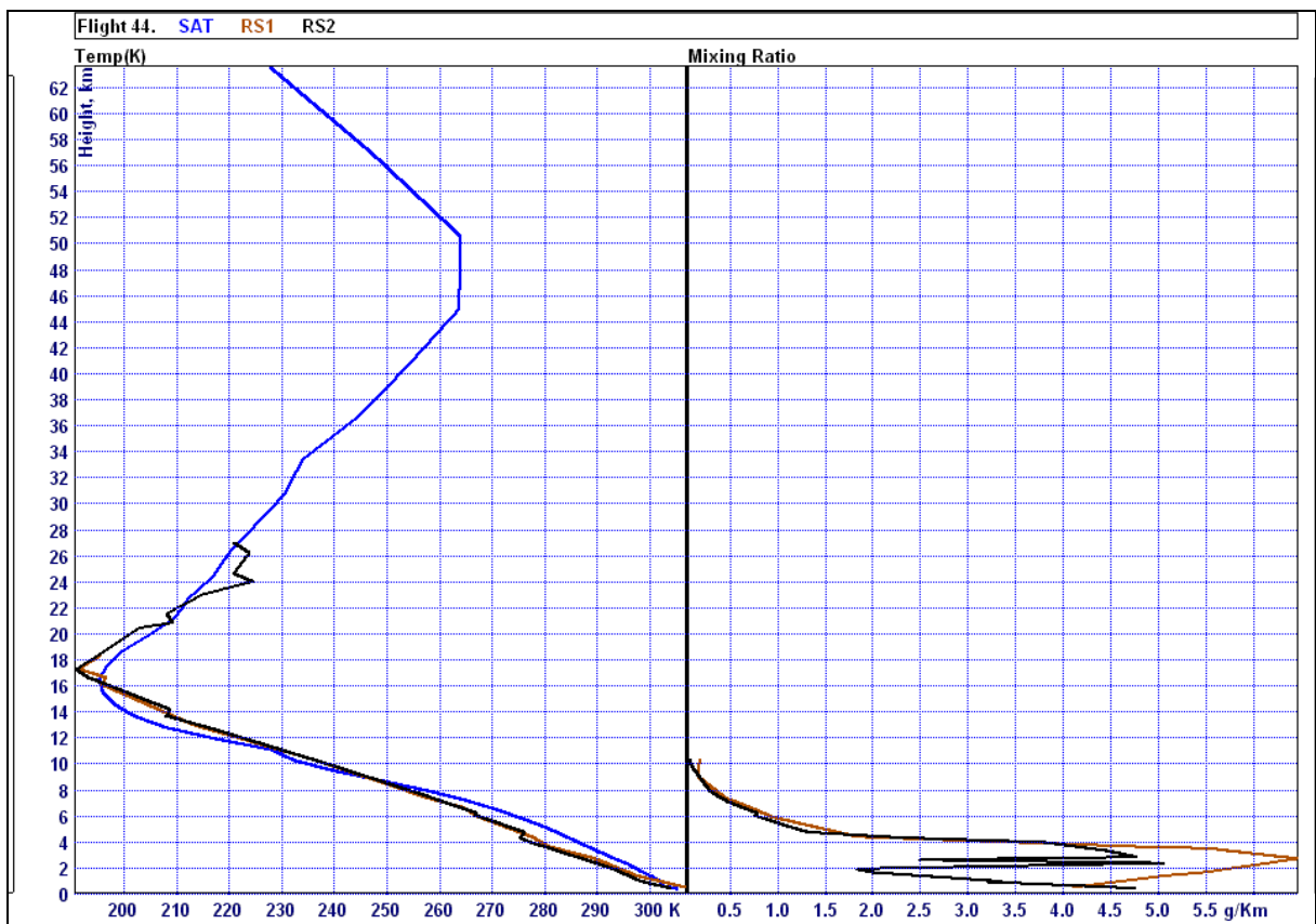
Figure E4 comparison 44 satellite and radiosonde profiles
