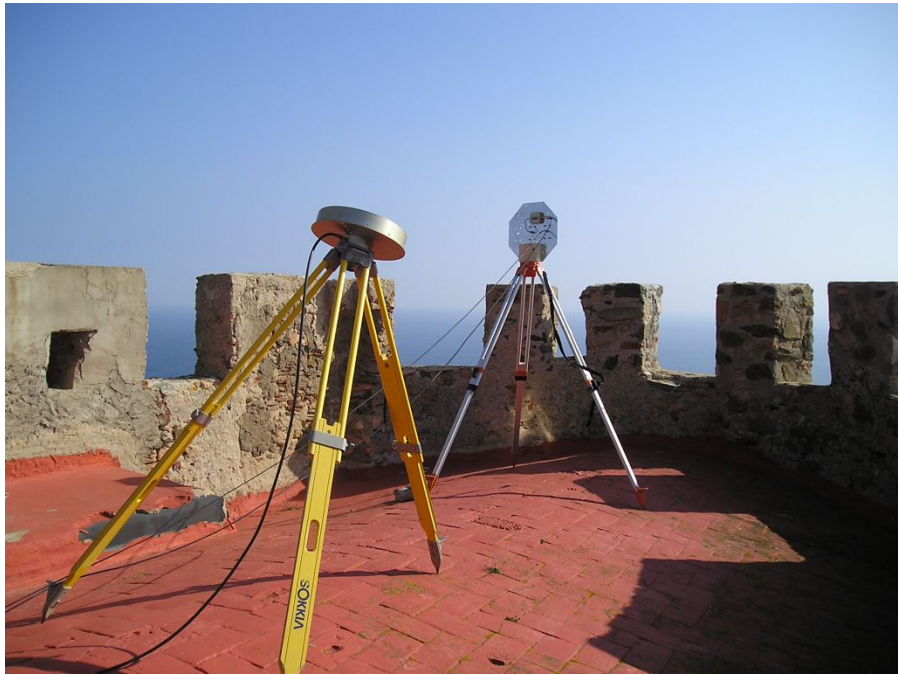
Figure 5.3: The antenna setup. In the front is the near zenith directed chokering antenna which feeds the ARS receiver. Behind is seen the metal plate on which the RHCP and LHCP antennas used for the raw sampling occultation measurements.
