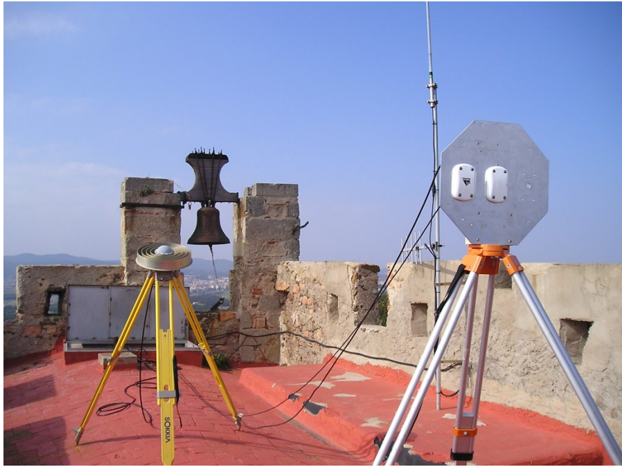
Figure 5.4: The antenna setup. In the back is the near zenith directed chokering antenna which feeds the ARS receiver. In front is seen the RHCP and LHCP antennas used for the raw sampling occultation measurements.
