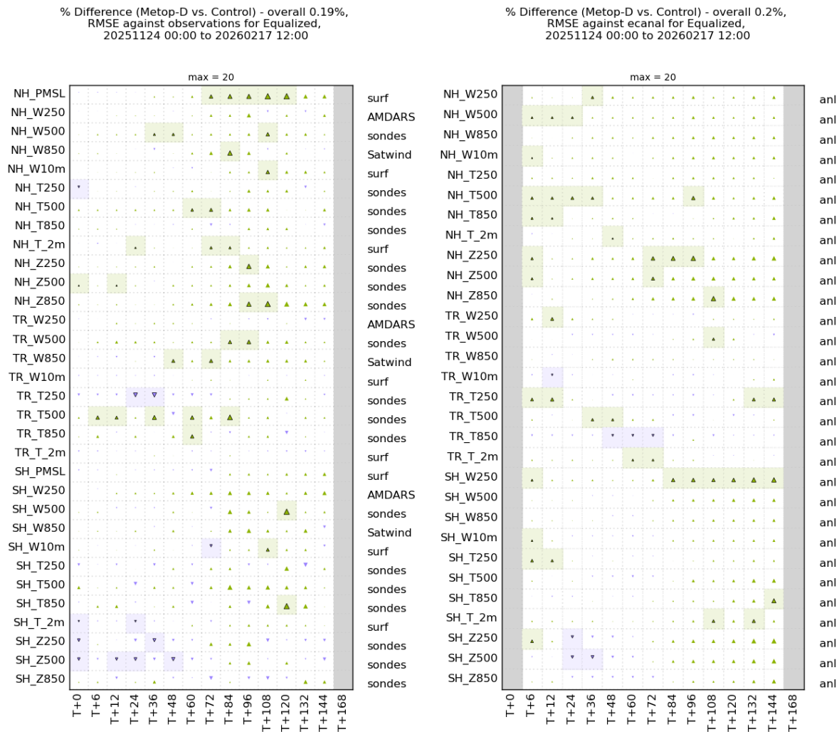
Figure 3.1: RMSE scorecards showing the impact of assimilating Metop-D data relative to the control, without Metop-D observations. This is for the period from 24th November 2025 to 17th February 2026. The left plot verified each trial against observations and the right plot verified against ECMWF analyses. PMSL, W, T and Z represent the pressure at mean sea level, wind vectors, temperature and geopotential height respectively. NH, SH and TR are Northern Hemisphere extratropics, Southern Hemisphere extratropics and Tropics, respectively. The scorecards are also separated by vertical levels in each region – NH_T500 which represents temperature in the Northern Hemisphere extratropics at 500 hPa. The forecast lead times are shown in hours (i.e. T + 24 is a 1-day forecast, T + 72 is a 3-day forecast and so on). Green (purple) triangles indicate improvements (degradations); triangle area represents impact magnitude and shaded squares denotes statistical significance.
