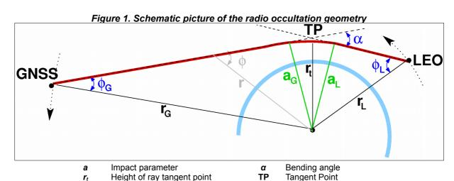
GNSS GNSS transmitter satellite LEO Low Earth Orbit receiver
