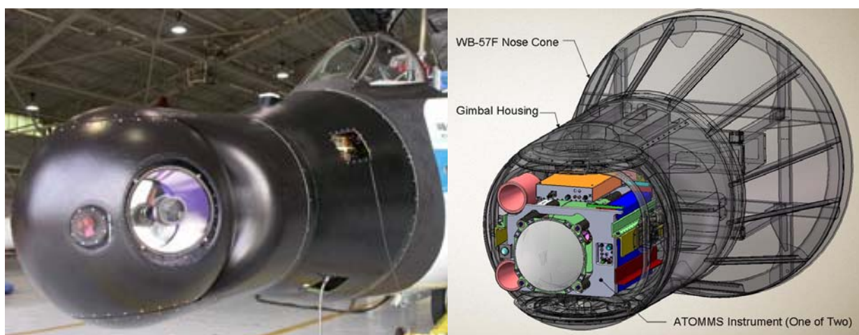
Figure 6: Left hand panel: WB-57F aircraft with gymbal nose cone. Right hand panel: ATOMMS instrument mounted in the nose cone gymbal.
